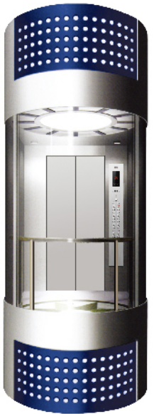
RJ105 (Standard) Car cover: Baked enamel steel frame, acrylic lighting decoration Observation wall: Laminated safety glass Decoration roof: Steel plate baked enamel frame, acrylic roof lamp with down lights Car wall: Hairline stainless steel Handrail: Stainless steel tube Floor: PVC
