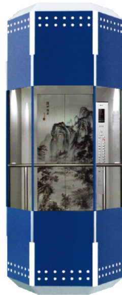
RJ108 (Optional) Car cover: Baked enamel steel, acrylic lighting decoration Observation wall: Laminated safety glass Decoration roof: Baked enamel steel frame, acrylic arch top plate with down lights Car wall: Hairline stainless steel Handrail: Stainless steel, single tube fixed on floor Floor: PVC
