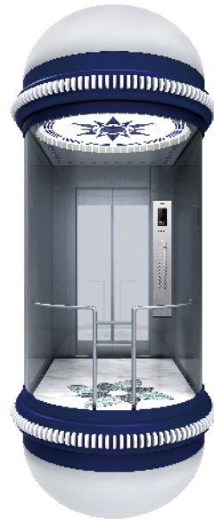
RJ102 (Optional) Car cover: White acrylic decoration hood Observation wall: Laminated safety glass (three pieces) Decoration roof: Baked enamel steel frame and blue acrylic lighting strip Car wall: Hairline stainless steel Handrail: Stainless steel tube Floor: PVC
